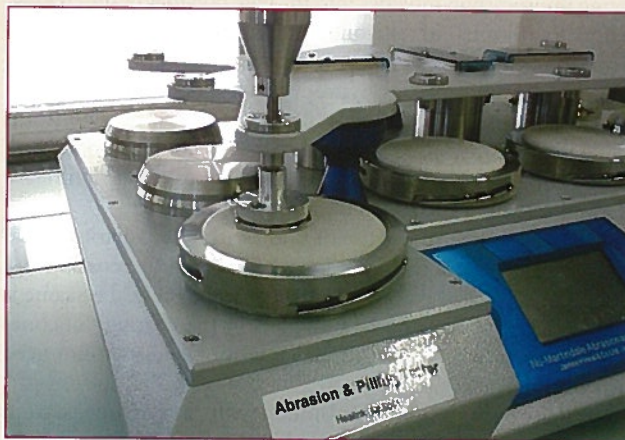
Item 1/2: Dynamic test, with Martindale equipment.
