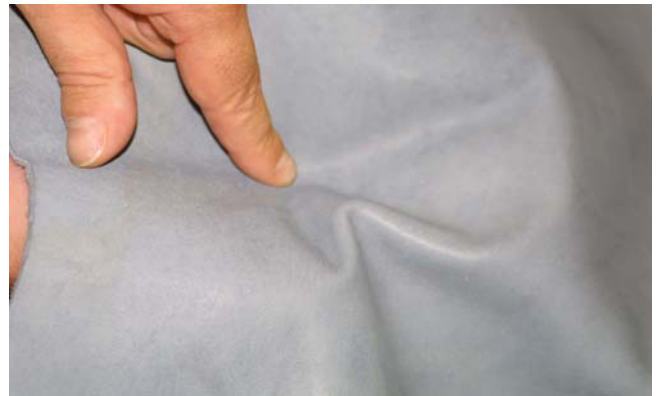
Grain tightness comparison of a proteolytic bacterial protease (left) versus modified OROPON bating product.
