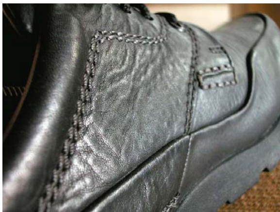
Loose leather parts used in articles. OROPON helps to improve layout but still keeps flanks full.
